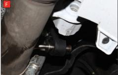
F) Replace the rear three moutuing rubbers with the uprated rubbers supplied in the fit kit.
