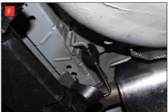
C) Remove the electronic actuator from the original exhaust.
