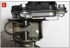
Before removing the original system disconnect the exhaust valve.
